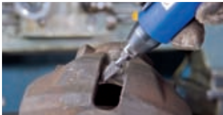
Tapered bur with radius end. PFERD Specification Number KEL
